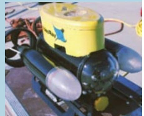
These robots are able to vacuum sediment from the floor of the tank while remaining on line and in service. A robotic camera is then deployed to inspect the tanks interior coating and structure to determine if repairs are needed.
